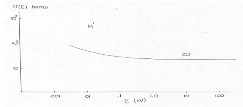
**Fig. 8.1.** Experimental neutron scattering cross section of hydrogen, showing a constant value of 20.4 barns over a wide range of neutron energy. The rise in the cross section at energies below  $\sim 0.1$  eV can be explained in terms of chemical binding effects in the scattering sample.
